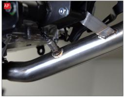
AO) Plug the lambda sensor into the extension cable and clip the cable back in place.
